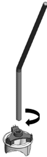
Figure 4. Schematic representation of cutting the attachment points of the prosthesis to holder for its removal with the aid of the holder.
